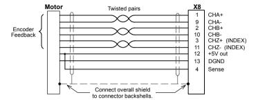
Figure 15 - Encoder cable connections without halls - rotary motors
